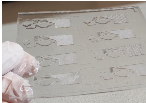
Roll-to-roll manufacture on polymer for high-volume, low cost manufacturing
