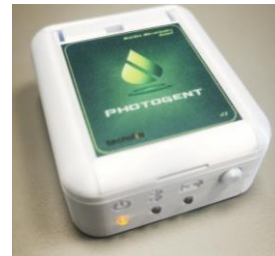
Small footprint colorimetric absorbance (405 and 570 nm) read-out device with integrated heating
