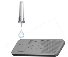
Microfluidic chip for measuring enzyme activity with colorimetric read-out device
