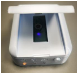
Small footprint colorimetric absorbance (405 and 570 nm) read-out device with integrated heating
