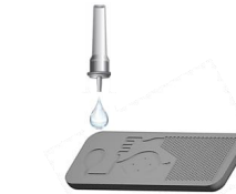
Transfer drop onto microfluidic chip inlet
